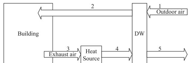
Fig. 1. Typical desiccant wheel system set-up.
