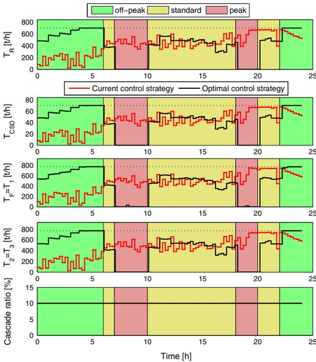
Fig. 5. Coal flow rates and cascade ratio.
