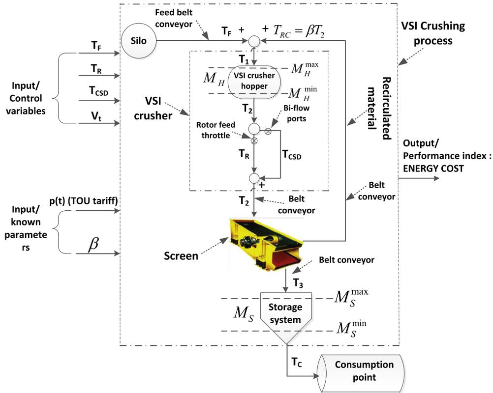
Fig. 1. Schematic of a tertiary mining VSI crushing station (adapted from [1]).
