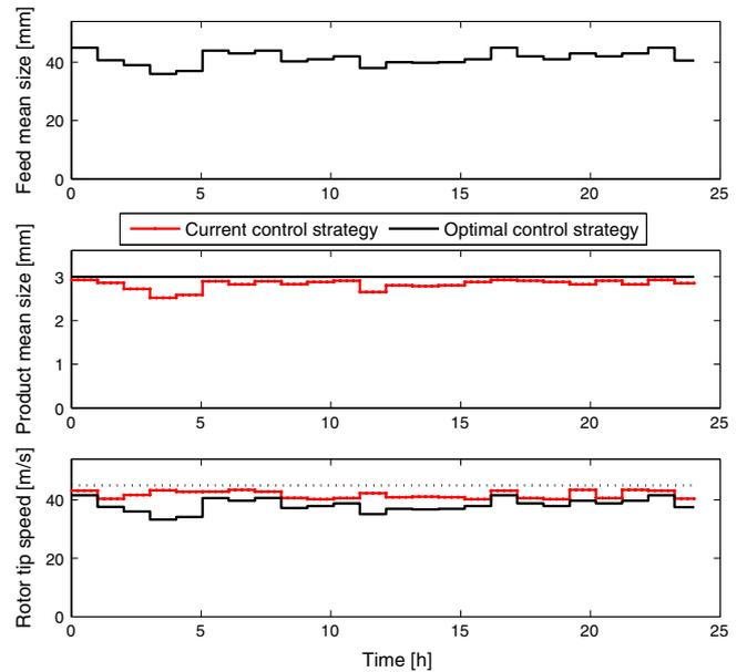
Fig. 7. Coal mean sizes and VSI crusher speed.
