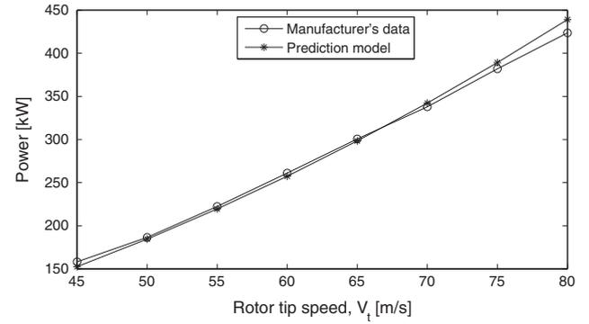
Fig. 3. Power curves for  $T = 300$  t/h.
