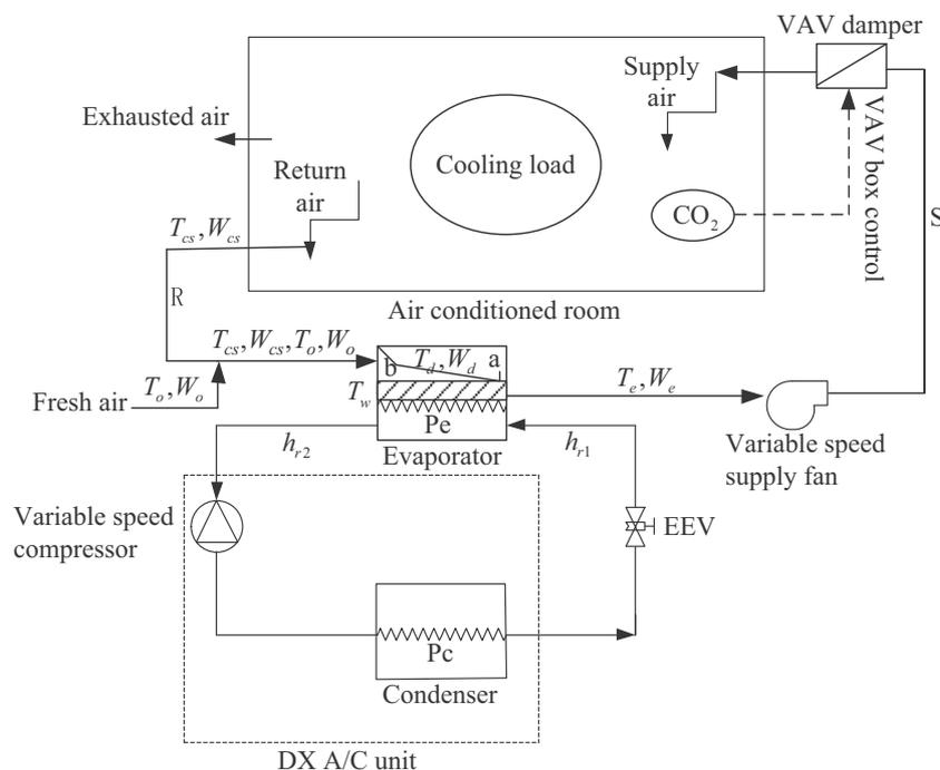
Fig. 1. Simplified schematic diagram of the DX A/C system.
