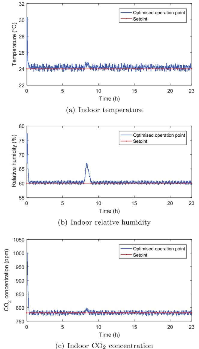
Fig. 11. The variation profiles of indoor temperature, relative humidity and CO<sub>2</sub> concentration of disturbance rejection capability test in the case of 25% exhausted air volume.
