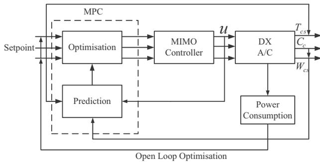
Fig. 5. Schematic diagram of the MIMO MPC with optimal control system.
