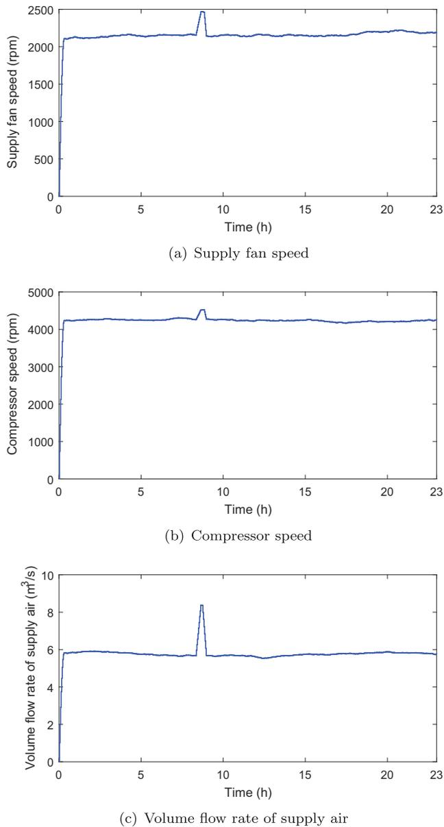
**Fig. 12.** The variation profiles of supply fan speed, compressor speed and volume flow rate of supply air of disturbance rejection capability test in the case of 25% exhausted air volume.
