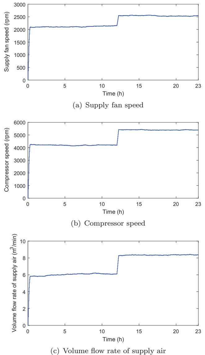
Fig. 9. Supply fan speed, compressor speed and volume flow rate of supply air for closed-loop system based on reference following in the case of 25% exhausted air volume.
