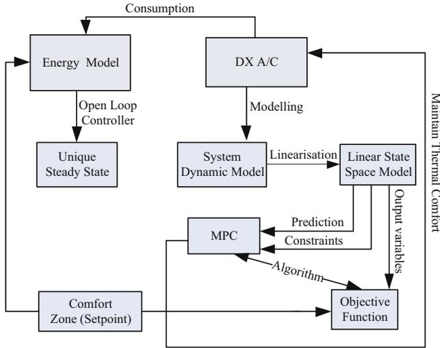
Fig. 4. Simplified flowchart of the proposed method.
