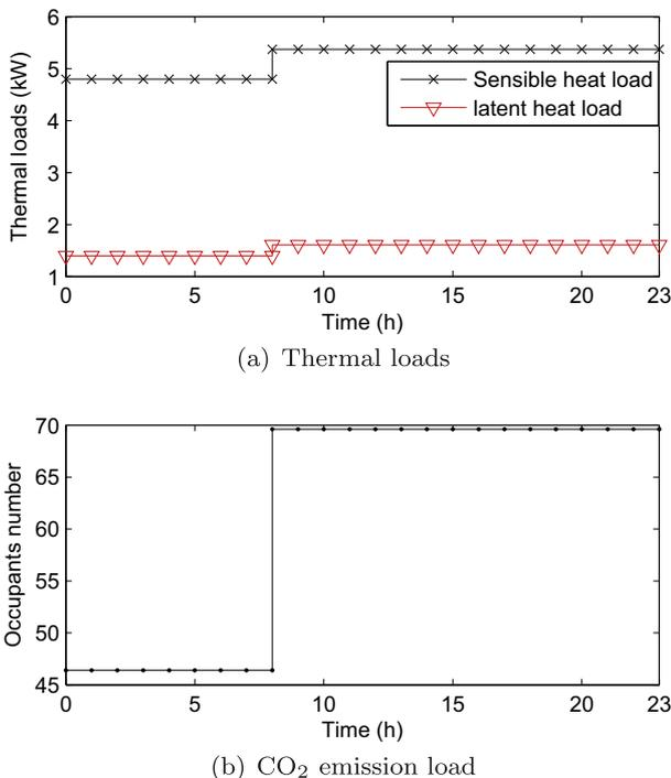
Fig. 10. The variation profile of thermal and CO<sub>2</sub> emission loads of disturbance rejection capability test in the case of 25% exhausted air volume.
