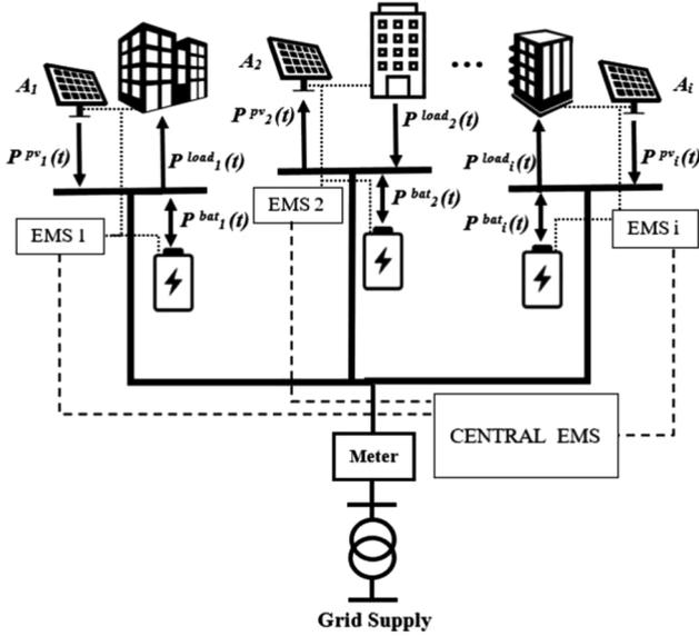
Fig. 4. An illustration of the user owned BESS with P2P energy sharing structure realisation.
