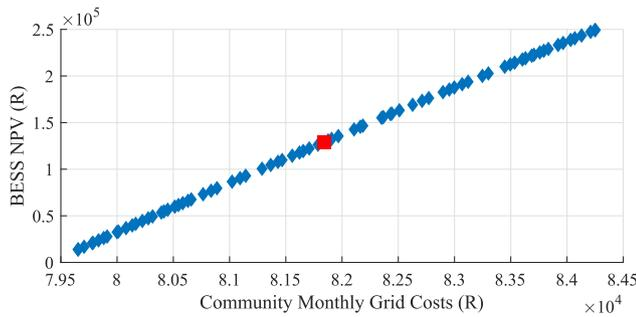
Fig. 12. Plot showing the simulation Pareto front for the community energy costs versus BESS NPV. The red square is the median point.
