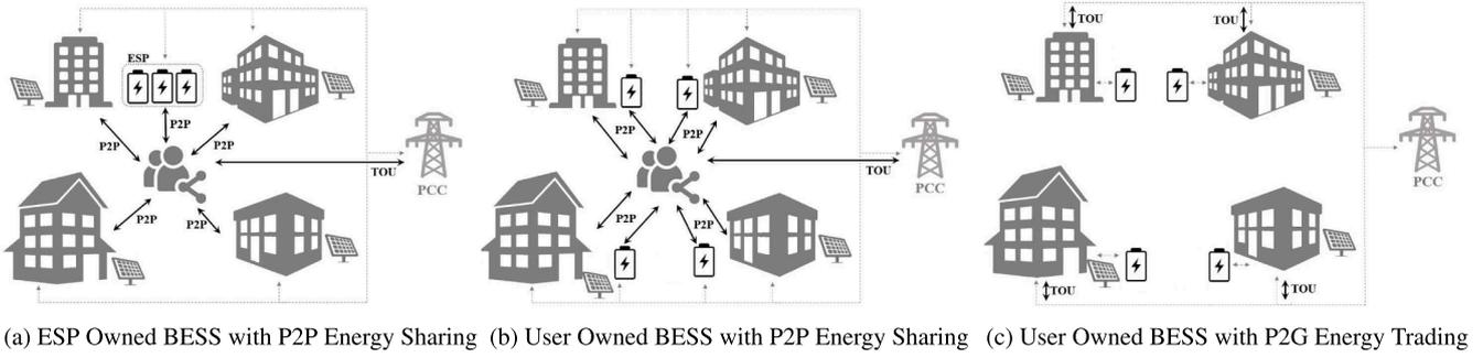
Fig. 1. BESS ownership structures; ESP with P2P energy sharing (a), User with P2P energy sharing (b) and User with P2G energy trading (c).
