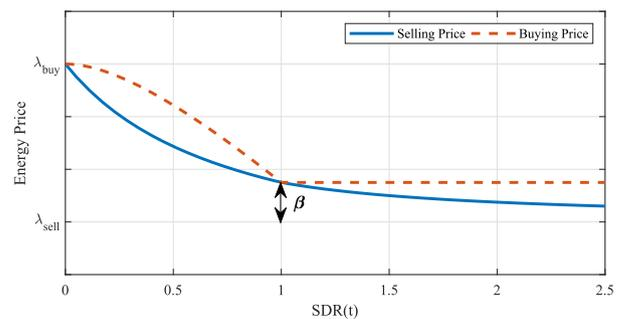
Fig. 3. The internal dynamic pricing with a compensating factor [6] as a function of SDR based from economics for prosumers in a P2P energy sharing community [18].
