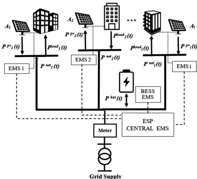
Fig. 2. An illustration of the ESP owned BESS structure with P2P energy sharing.
