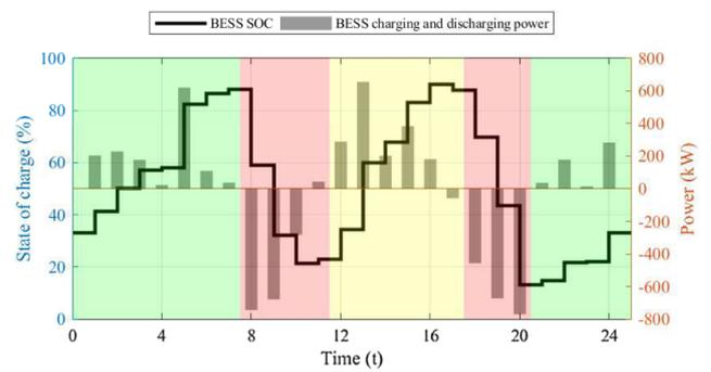
Fig. 7. BESS SOC, charging and discharging power.
