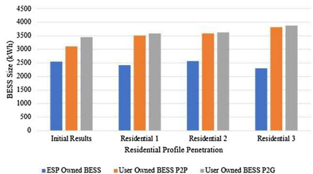
**Fig. 17.** BESS size against residential profile penetration.
