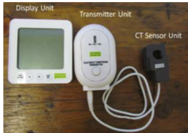
Fig. 2. Efergy E2 Classic energy monitor components.
