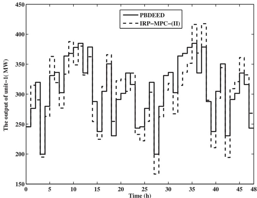
Fig. 11. The generation output of the six-unit system under PBDEED for  $\alpha = 0.7$ , price-II and IRP-MPC-(II).
