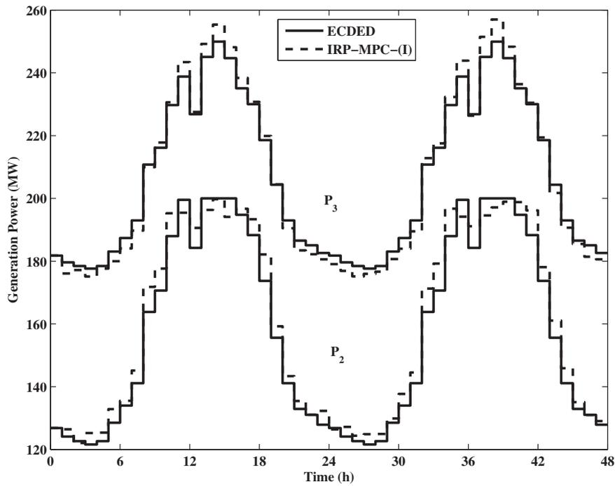
Fig. 4. The generation output of the six-unit system under ECDED and IRP-MPC-(I).
