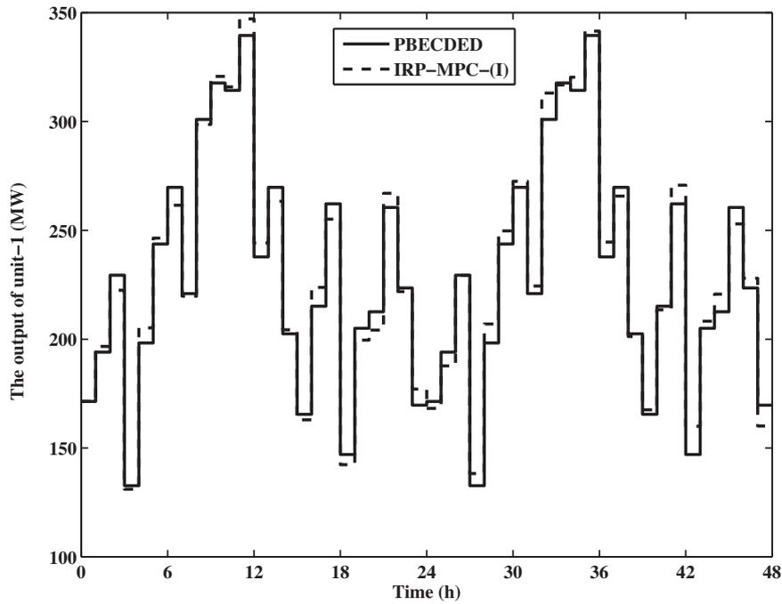
Fig. 10. The generation output of the six-unit system under PBECEDED for  $E^{\max} = 16, 200$  lb, price-II and IRP-MPC-(I).
