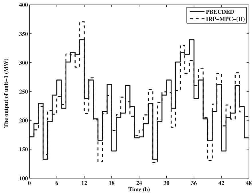
Fig. 12. The generation output of the six-unit system under PBECEDED for  $E^{\max} = 16, 200$  lb, price-II and IRP-MPC-(II).
