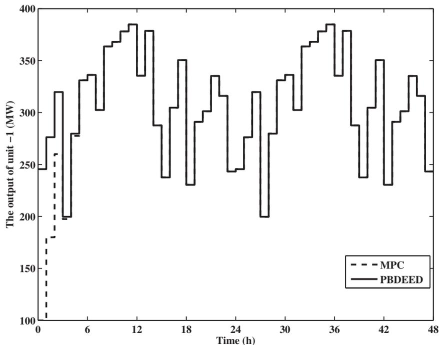
**Fig. 7.** Convergence of the MPC solution of the six-unit system to those of PBDEED for  $\alpha = 0.7$  and price-II.
