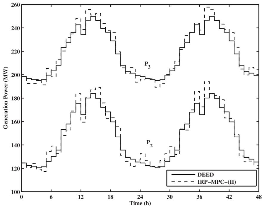
Fig. 5. The generation output of the six-unit system under DEED and IRP-MPC-(II).
