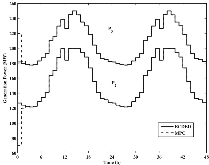
Fig. 2. Convergence of the closed-loop MPC solutions to those of ECDED for the six-unit system.
