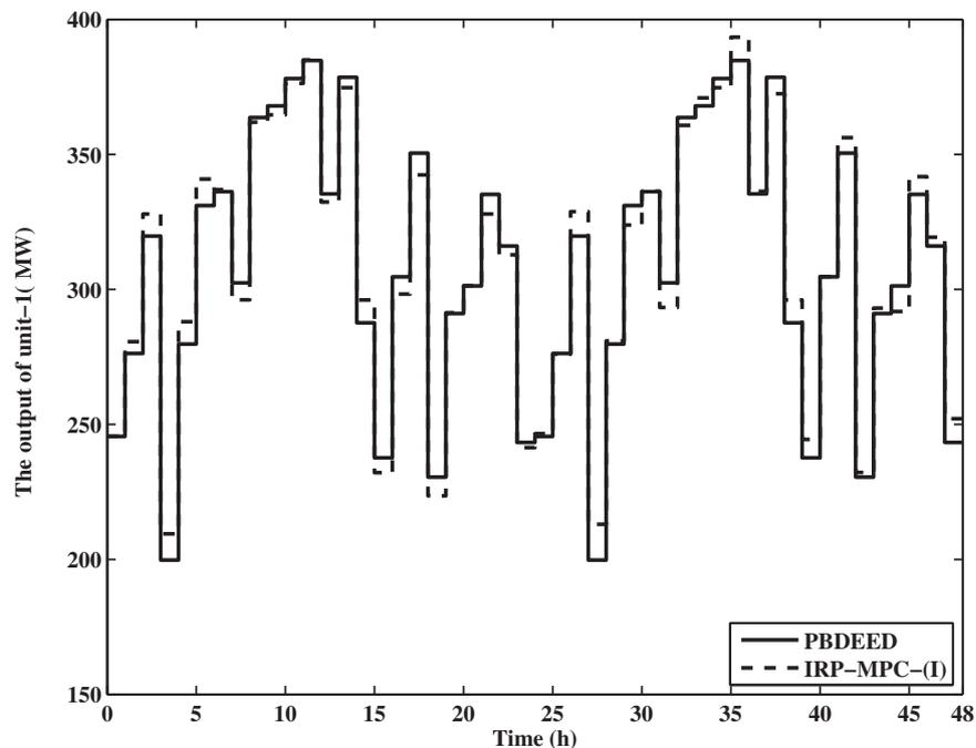
Fig. 9. The generation output of the six-unit system under PBDEED for  $\alpha = 0.7$ , price-II and IRP-MPC-(1).
