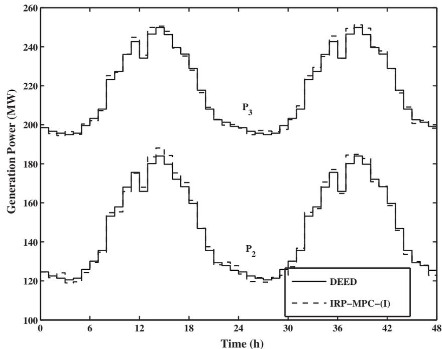
Fig. 3. The generation output of the six-unit system under DEED and IRP-MPC-(I).
