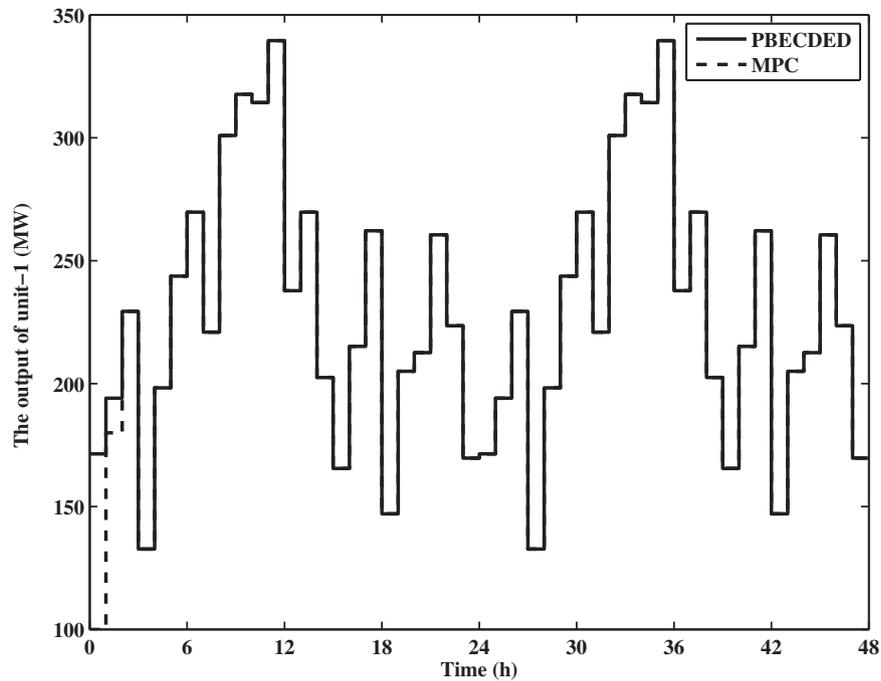
Fig. 8. Convergence of the MPC solution of the six-unit system to those of PBECEDED for  $E^{\max} = 16, 200$  lb and price-II.
