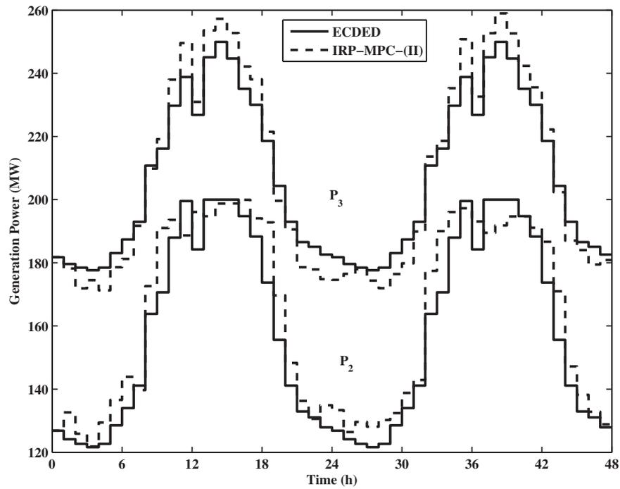
Fig. 6. The generation output of the six-unit system under ECDED and IRP-MPC-(II).
