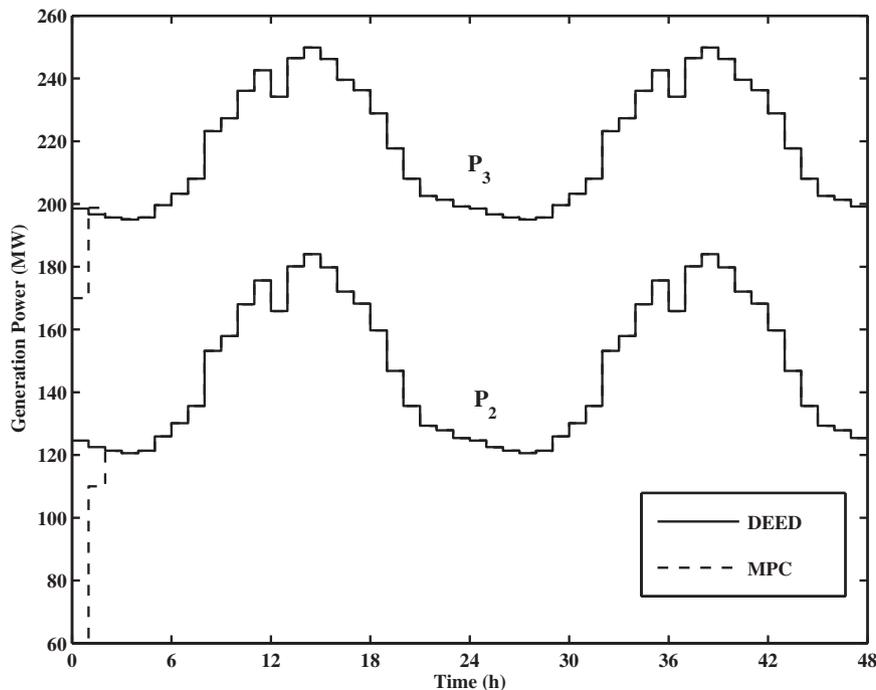
**Fig. 1.** Convergence of the closed-loop MPC solutions to those of DEED for the six-unit system.
