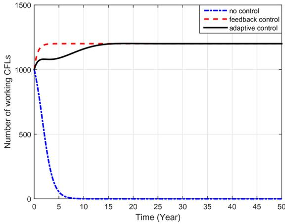
Fig. 2 Performance of controller design ( $k_1 = 1.5$  and  $k_2 = 0.5$ )
